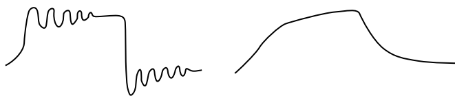
RESET OR RATE TOO HIGH RESET OR RATE TOO LOW Figure 7. Setting RESET and/or RATE
