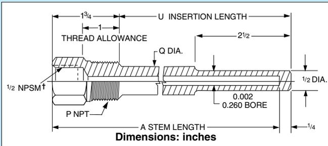
† NPSM internal pipe thread will accept both NPT and NPS male threads.
