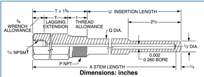
† NPSM internal pipe thread will accept both NPT and NPS male threads.
