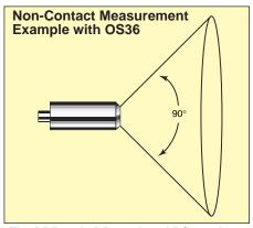
The DP5000A, B56000A and BS6001A can be used with infrared sensors for non-contact temperature measurements. Fields of view range from 90 to 0.06°.
