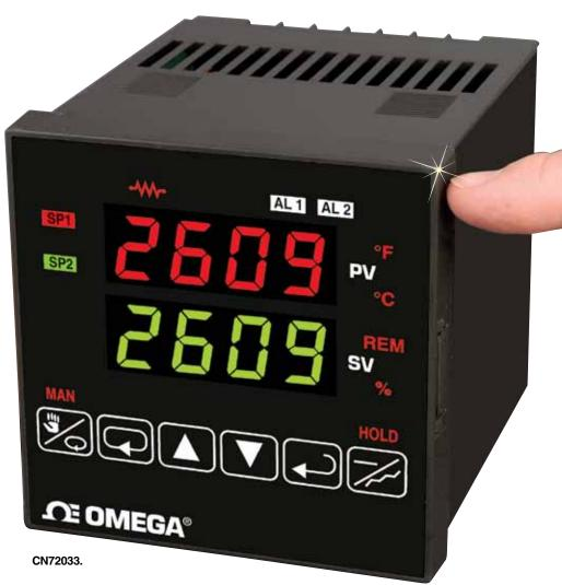
RTD inputs show whole or tenth degree displays. The CN72000 Series can be programmed for on/ off, PID, heat/cool, or latching alarm. All outputs are isolated from the inputs. Outputs include 10 A relay, and scalable 0 to 20 mAdc.
