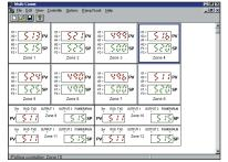
Sample of screen displaying status of multiple controllers.
