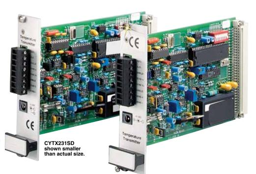
Electronic Accuracy: CYTX231SD,  $\pm 0.07$  K at 4.2 K: CYTX231P  $\pm 0.15$  K at 77 K
