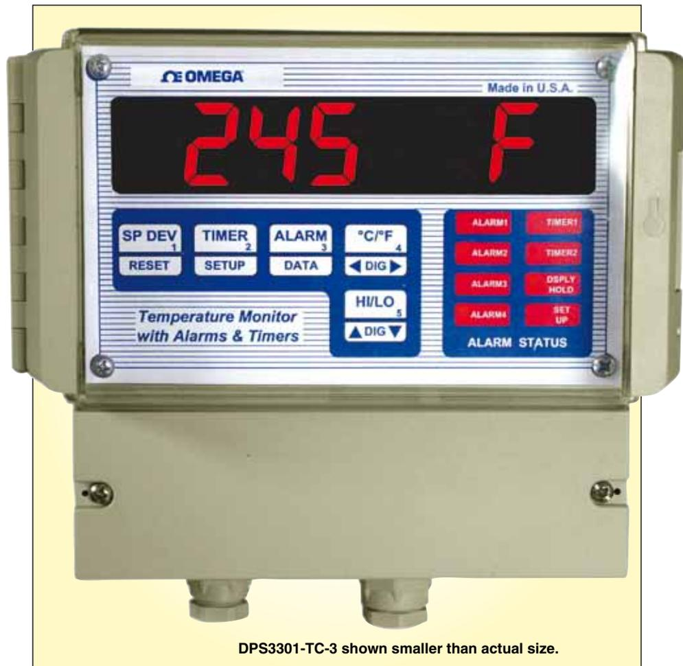
Four (optional) process alarms are available that are programmable over the entire range of selected input type. They can be configured as latching or non-latching, normally open, or normally closed. Also available are 2 optional timers that work independently or in conjunction with process limits (e.g., turning on a fan 10 minutes after limit 1 temperature is reached). The time function keeps track of process run time.
