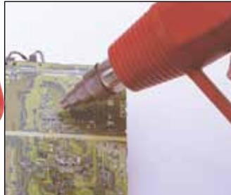
HG1500 heat gun being used to desolder an electronics board.
