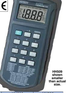
**Specifications HH508 HH509 Backlit LCD** No. of Digits 1999 1999 K/J/E/T/S Probe (Type) K/J/E/T/S Input Channel -210 to 1767°C -210 to 1767°C Range °C Range °F -346 to 1999°F -346 to 1999°F 0.1°/1° 0.1°/1° Resolution Data/Hold Max/Min • Relative Hi/Lo Limits w/Beeper Warning **Display** 1 1 T1-T2 **Battery (included)** 9V 9V **RS232C Auto Power-Off** 0.1% +1°C **Basic Accuracy** 0.1% 1°C
