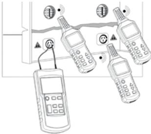
Locating a socket, switch, junction box or fuse, or tracing a line
