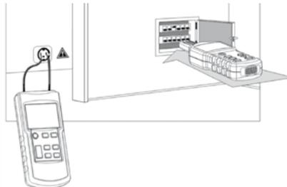
Identifying the fuse or circuit breaker associated with an AC outlet
