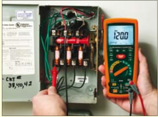
Only a True RMS meter can give accurate readings of distorted waveforms.
