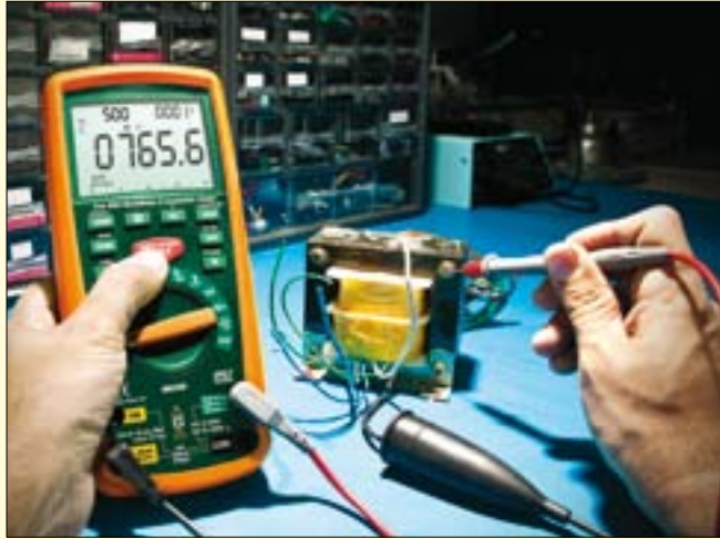
Measure the insulation resistance of transformer windings
