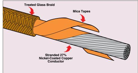
HTMG high-temperature lead wires are designed for appliances and industrial heating products—such as commercial food service equipment, heaters, heat treating furnaces, kilns, heater elements and other applications up to 450°C (842°F).
