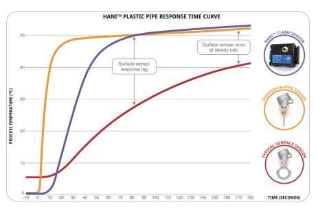
1.  $\tau_{63}$  is the time constant or response time required to reach 63.2% of the final value after an instantaneous temperature change.  $\tau_{90}$  is the response time required to reach 90% of the final value after an instantaneous temperature change.
