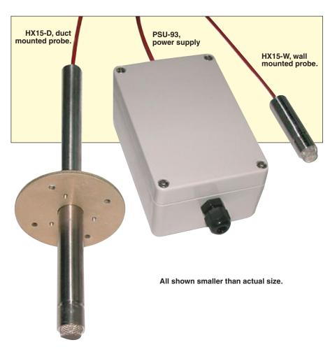
Sensors: RH, thin polymer capacitor; temperature,  $1000 \Omega$  Platinum RTD
