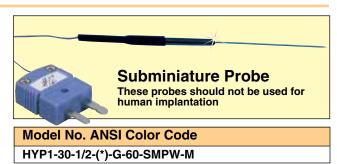
\* Specify calibration: **K**, **T**, or **E**. K = CHROMEGA®-ALOMEGA®, T = Copper-Constantan, E = CHROMEGA®-Constantan For lead wire lengths over 1.5 m (60") at an additional cost/300 mm (12") and modify model number.
