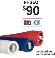
The OMEGALUX® PHSEQ connects to any 3-phase circuit from 115 to 700 V. The test leads follow an easy-to-remember red, white, and blue "ABC" color code. Proper phase sequence will illuminate the "ABC" lamp. A reversed sequence will illuminate the "BAC" lamp, and an open-phase condition will illuminate both lamps.
