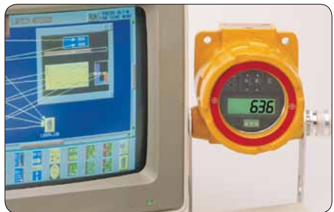
Standard 4 to 20 mA output can be used with data acquisition equipment for computer-based monitoring and control.
