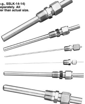
OMEGA® miniature and standard protection tubes are available in 316 stainless steel and Inconel 600 nickel alloy. Tubes are available either opened at both ends or with one end closed. Standard length available from stock is 150 mm (6"); however, practically any length tube is available on short delivery.
