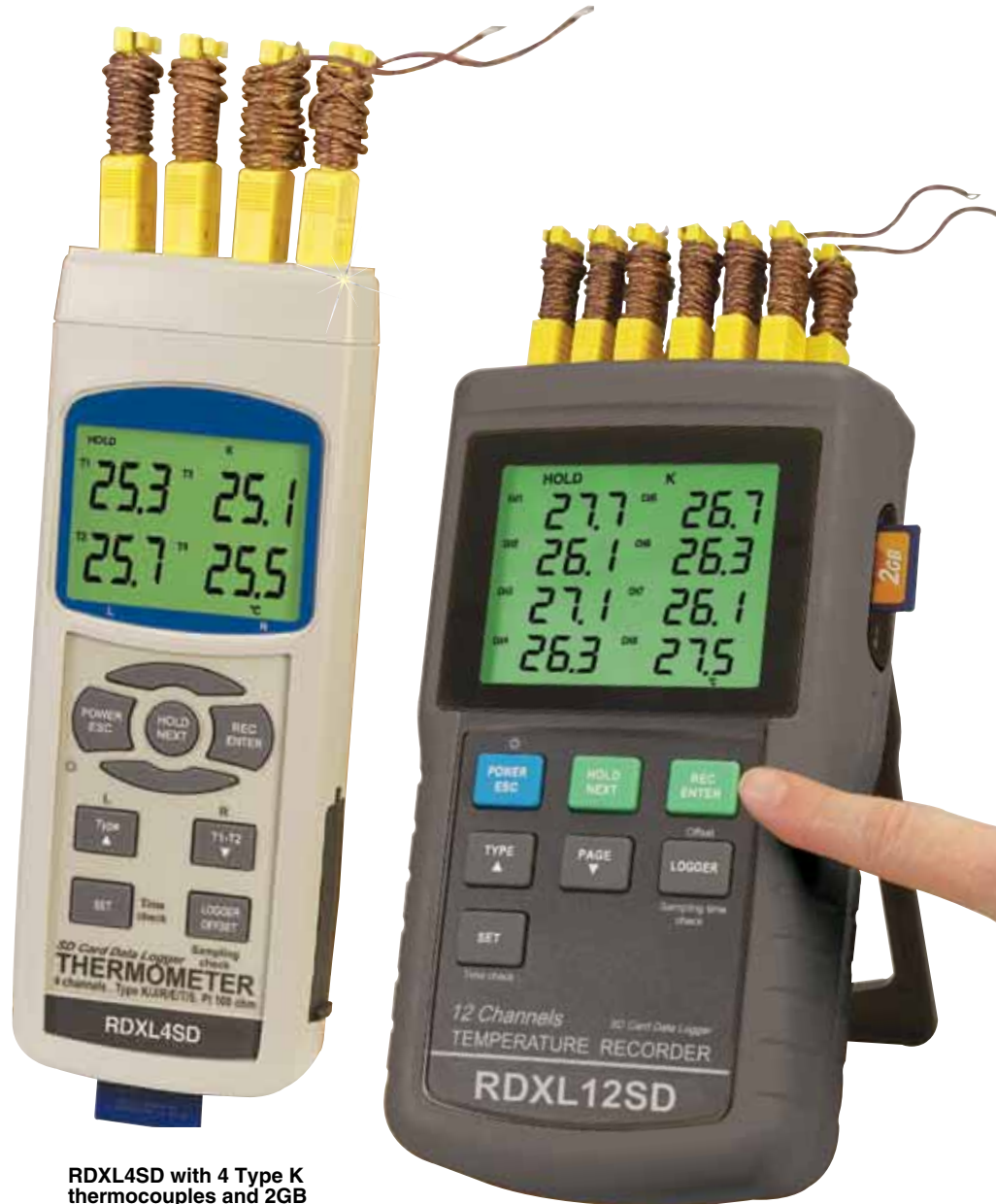
RDXL12SD with 12 Type K thermocouples and 2GB SD memory card (included).
