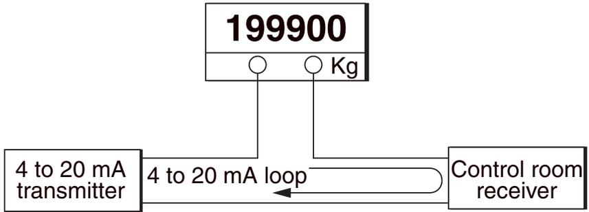
A TX82B process-loop indicator may be added to an existing 1 to 5 mA, 4 to 20 mA or 10 to 50 mA installation to provide a local readout scaled in percent or engineering units. No power wiring is required, since the meter is powered directly by the current loop.
