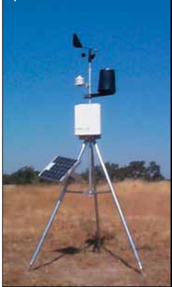
WMS-16NEMA-S, modular weather station with NEMA enclosure and solar power.
