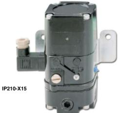
Zero adjustment of the unit is made by turning a screw that regulates the distance between the flapper valve and the air nozzle. Span adjustment is made by varying a potentiometer, which shunts input current past the coil. An integral volume flow booster provides adequate flow capacity, resulting in fast response time and accurate control.
