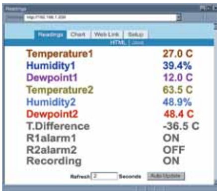
Readings through embedded Web server
